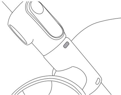
1.1 Your Wayfarer cup holder can be attached to either side of your Wayfarer pushchair handle. Attach your Wayfarer cup holder by clipping the cup holder clamp to your Wayfarer chassis on the lower part of the handle, ensuring your cup holder is the correct way up.
